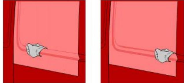
10. With all the edges properly applied, it is necessary to apply the material in the center of the corrugation. When doing this make sure that the air is not trapped, always leave an opening for the air to escape.
