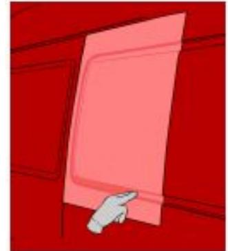
11. Check the application for remaining bubbles. If there still are small air bubbles to be seen, these can easily be removed. Just make a small puncture, heat it (40-50 °C) and push the air out.
