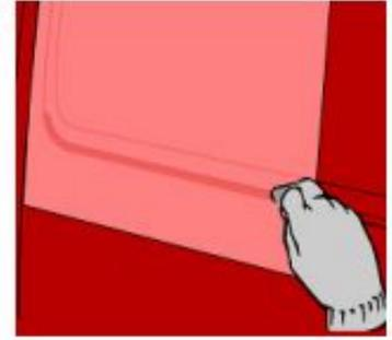
9. When all the deepest areas of the corrugation have been applied, the remaining part of the corrugation can be done. Again, make sure the material is heated to the required 40°-50°C, and work you way through the corrugation.
