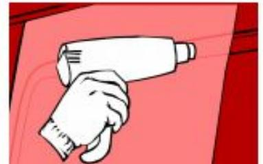
7. Now, start stretching the material in the corrugation, starting in the deepest part of the corrugation first (the part where the material will require the most amount of stretch, such as a corner). Make sure that the material is heated to remain at the 40°-50°C temperature.
