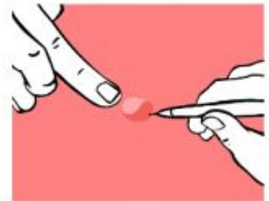
12. The final stage of the application starts. Using the hot air gun, the material should be post heated to a temperature of 90-95°C, especially in those areas where the material is stretched. The use of an AD laser temp is REQUIRED to ensure you achieve the proper temperature during the post heating process. Make sure that the heating is done gently, and the temperature is gradually increased.
