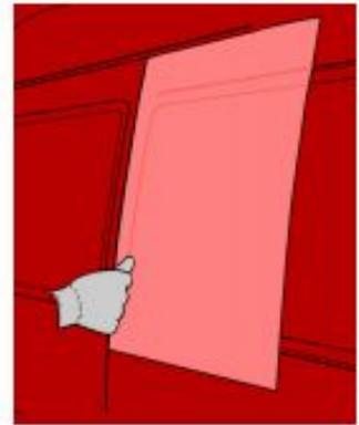
5. Now the application of the material in the corrugation can start. In order to be able to do so without forming wrinkles or creases, it is advised to wet the AD application glove, using a water/soap mixture.
